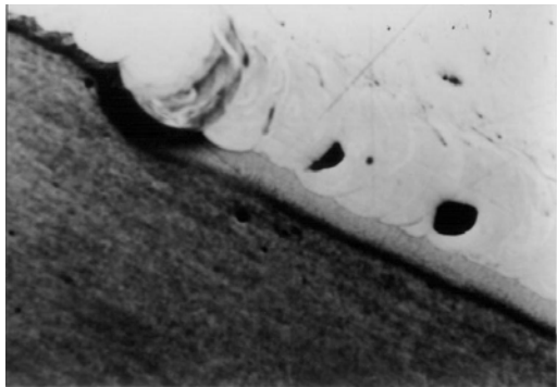
Fig. 10 Macrostructure of the weld with welding energy of 6.38 J, welding rate is changed from 1.35 mm/s (above) to 1.80 mm/s (below); increased 25 times
