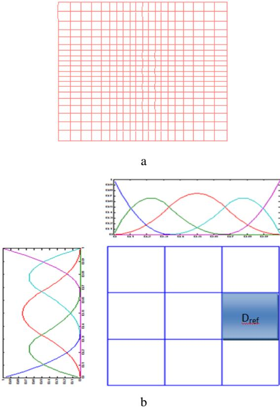
Fig. 5 a - Geometry of the model obtained by second order NURBS functions; b - parameter space associated
