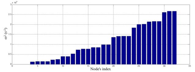
Fig. 6 Eigenvalues of the thin plate using first order NURBS functions
