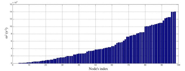
Fig. 7 Eigenvalues of the thin plate using second order NURBS functions
