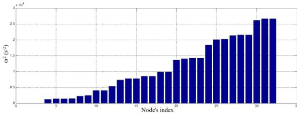
Fig. 2 Eigenvalues of the thin plate using Q4 Lagrange elements
