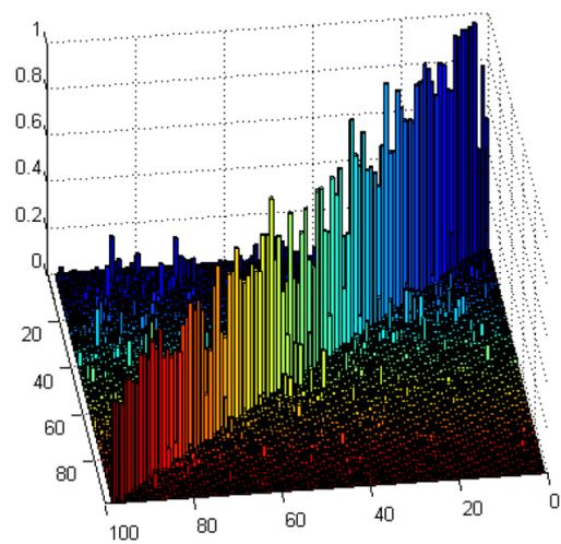
Fig. 9 MAC matrix obtained from the eigenmodes given by second order Lagrange and NURBS functions
