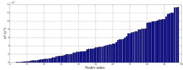
Fig. 3 Eigenvalues of the thin plate using Q9 Lagrange elements
