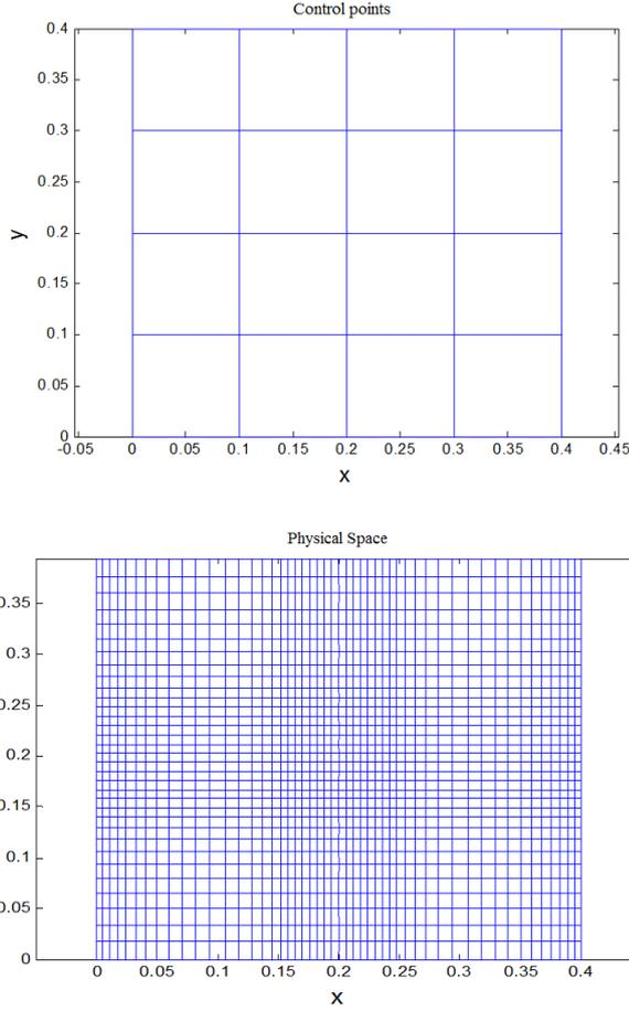
Fig. 1 Control points and NURBS geometry of a thin plate
