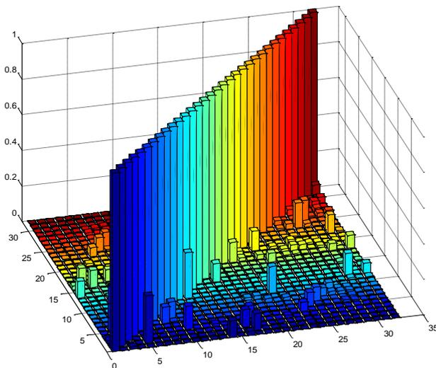
Fig. 8 MAC matrix obtained from the eigenmodes given by first order Lagrange and NURBS functions
