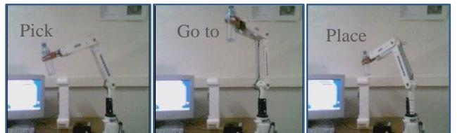
Fig. 6 Realisation of the pick-and-place task by the manipulator arm
