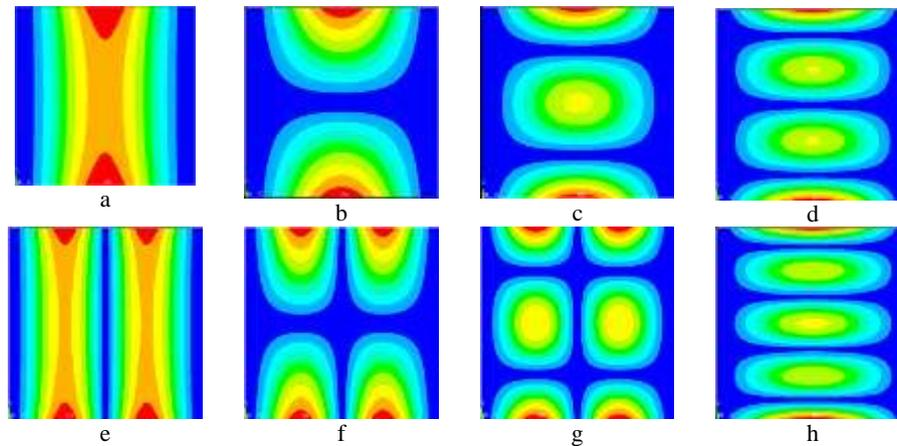
Fig. 2 Calculated mode shapes: (a–h) – 1 to 8 modes respectively
