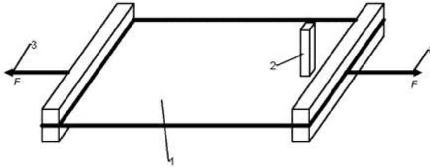
Fig. 1 Scheme of test equipment: 1 – print or paper; 2 – piezoelectric transducer; 3 – tension direction
