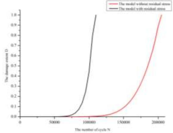
Fig. 15 The change of damage extent versus number of cycles
