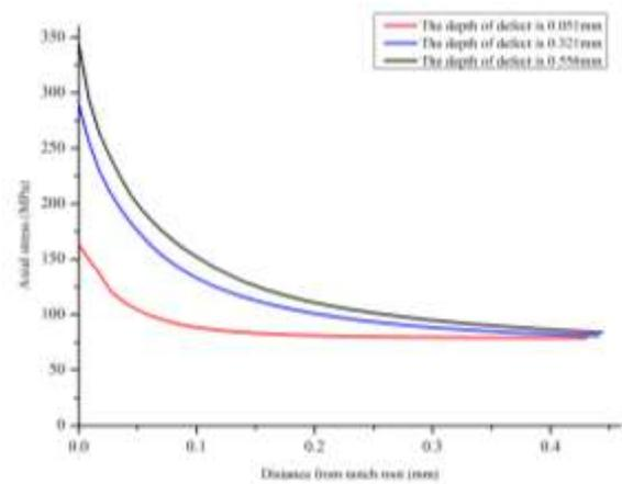
Fig. 10 Axial stress inward from the notch root when  $\sigma_{n,max} = 80$  MPa
