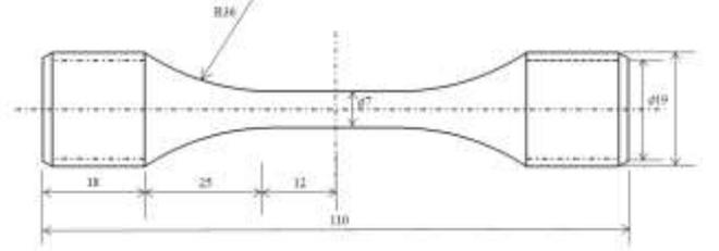
Fig. 1 Smooth specimen geometry (dimensions in mm)
