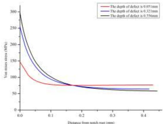
Fig. 11 Von Mises stress inward from the notch root when  $\sigma_{n,max} = 80$  MPa
