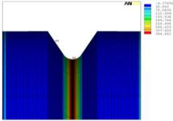
Fig. 8 Distribution of axial stress in the undamaged state
