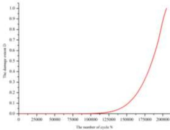
Fig. 9 The change of damage extent versus number of cycles
