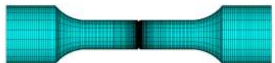
Fig. 7 The actual FE mesh of specimen with defect
