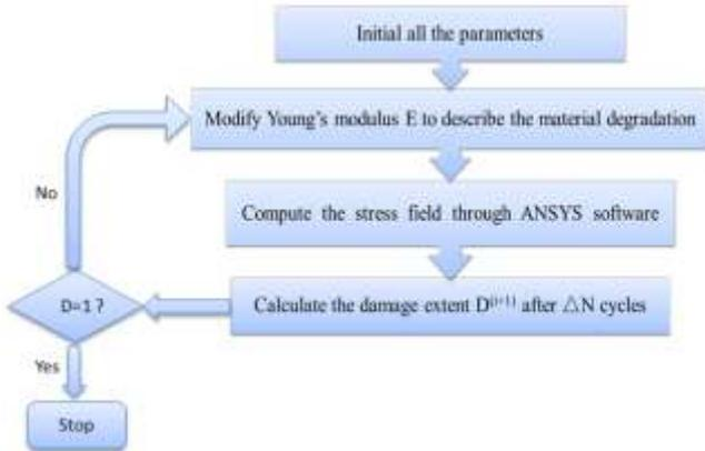
Fig. 3 The simplified FE computational methodology
