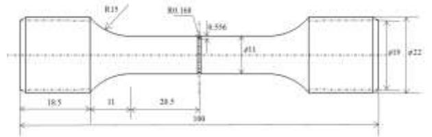
Fig. 4 Specimens with defect geometry (dimensions in mm)
