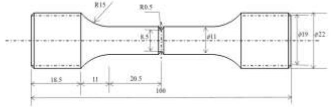
Fig. 2 Notched specimen geometry (dimensions in mm)
