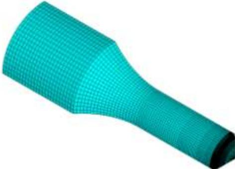
Fig. 13 The FE model after meshing
