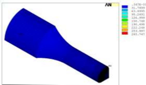
Fig. 14 Distribution of von Mises stress after cutting
