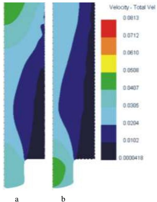
Fig. 15 Velocity distributions while forward extruding with motives parameters: a)  $R = 14 \mu\text{m}$ ,  $AR = 26 \mu\text{m}$ ; b)  $R = 5 \mu\text{m}$ ,  $AR = 17 \mu\text{m}$
