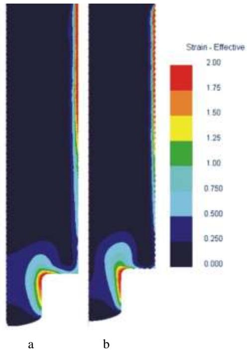
Fig. 14 Effective strain distributions while forward extruding with motives parameters: a)  $R = 14 \mu\text{m}$ ,  $AR = 26 \mu\text{m}$ ; b)  $R = 5 \mu\text{m}$ ,  $AR = 17 \mu\text{m}$
