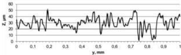
Fig. 4 Profile of the container roughness  $Ra = 3.5 \mu\text{m}$ , measured along an axis [6]
