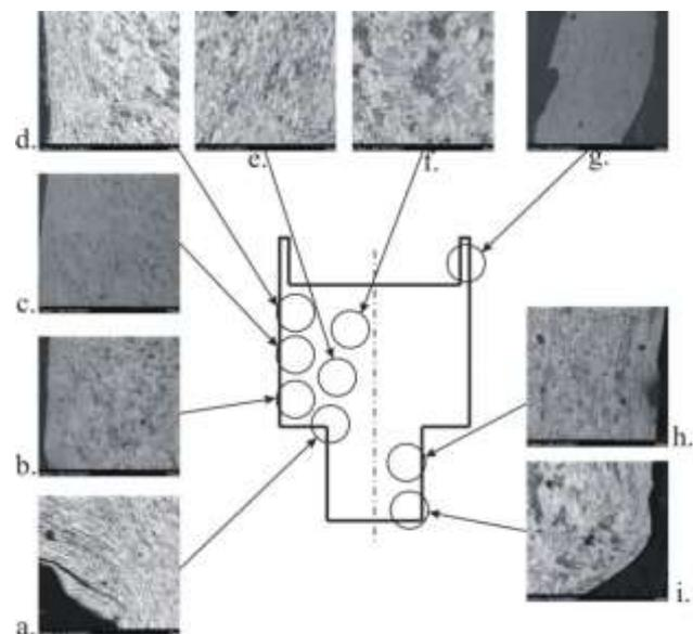
Fig. 7 Grain structure of forwardly extruded copper in a container with roughness  $Ra = 3.5 \mu\text{m}$ ; magn.  $\times 500$
