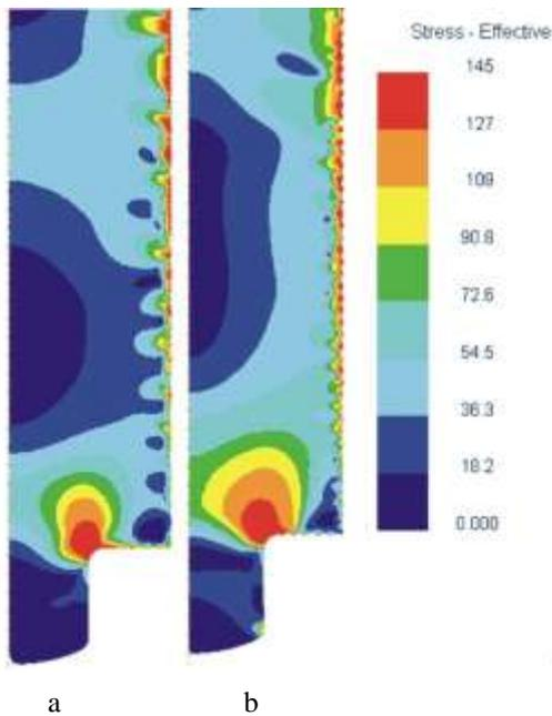
Fig. 13 Effective stress distributions while forward extruding with motives parameters: a)  $R = 14 \mu\text{m}$ ,  $AR = 26 \mu\text{m}$ ; b)  $R = 5 \mu\text{m}$ ,  $AR = 17 \mu\text{m}$
