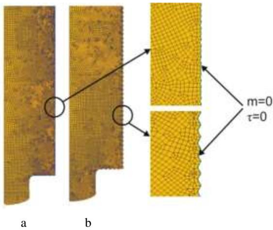
Fig. 12 Workpieces with the finite element mesh during extruding in the containers with roughness modeled in the form of triangle motives: a)  $R = 14 \mu\text{m}$ ,  $AR = 26 \mu\text{m}$ ; b)  $R = 5 \mu\text{m}$ ,  $AR = 17 \mu\text{m}$
