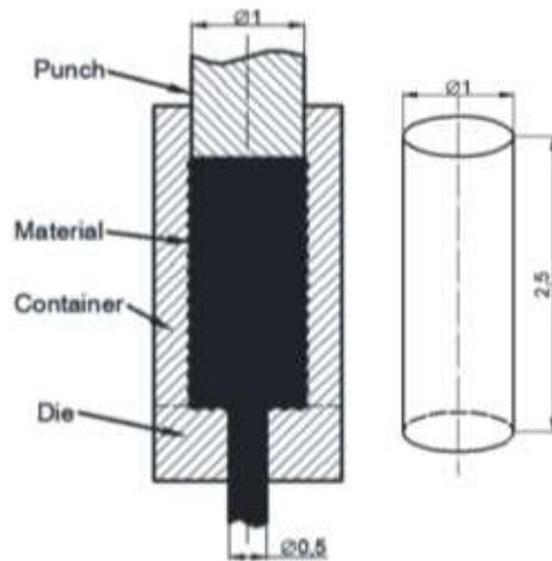
Fig. 10 Adopted for calculations model for forward micro-extrusion
