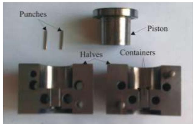
Fig. 1 View of the toolkit for forward microextrusion [6]
