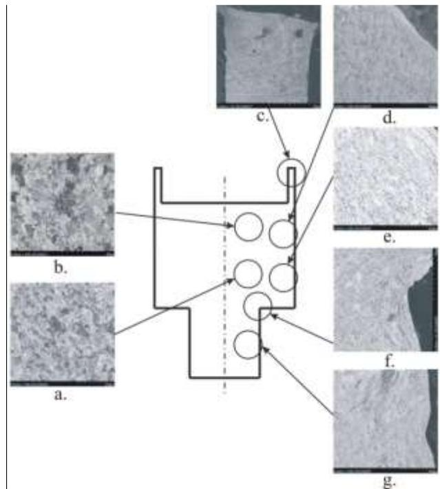
Fig. 6 Grain structure of forwardly extruded copper in a container with roughness  $Ra = 1.2 \mu\text{m}$ ; magn.  $\times 500$
