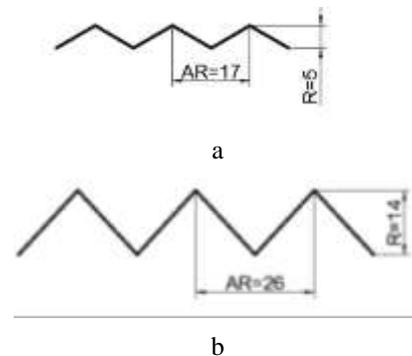
Fig. 11 Average profiles of containers roughness: a)  $Ra = 1.2 \mu\text{m}$ ; b)  $Ra = 3.5 \mu\text{m}$
