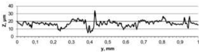
Fig. 3 Profile of the container roughness  $Ra = 1.2 \mu\text{m}$ , measured along an axis [6]
