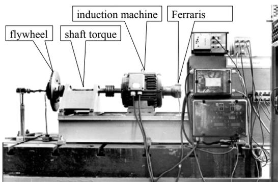
Fig. 8 Test rig to investigate torsional vibrations
