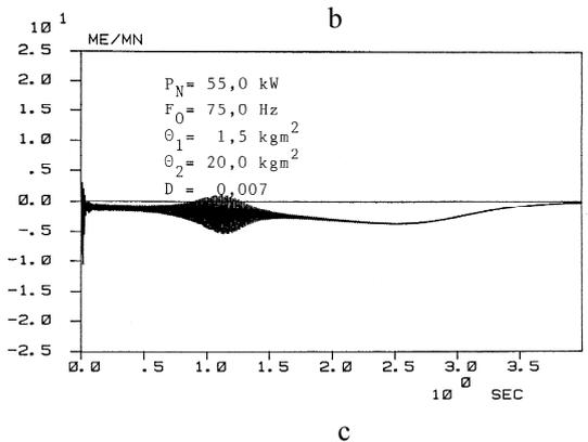
Fig. 5 a - parametric excitation of the shaft torque during reversal; b - simulation of the speed during reversal; c - simulation of electrical torque (reversal)
