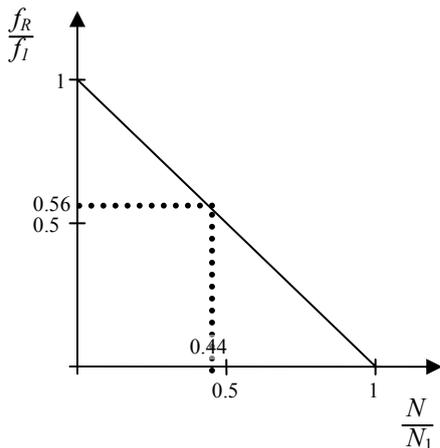
Fig. 4 Excitation condition diagram for run-up
