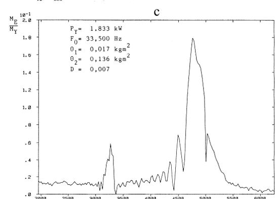
Fig. 9 a - measured parametric excitation of the shaft torque (run-up); b - measured speed (run-up); c - measured electrical torque (run-up); d - measured spectrum of the electrical torque (run-up)
