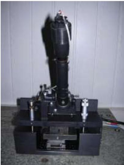
Fig. 11 SPM with nanomanipulator
