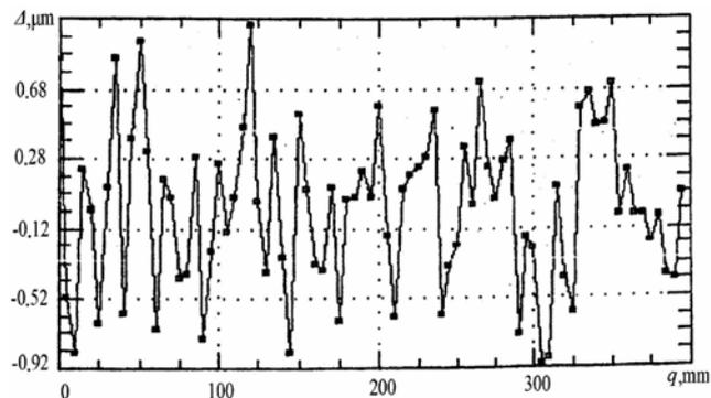
Fig. 6 Dependence of high frequency error of motion straightness on the displacement  $q$
