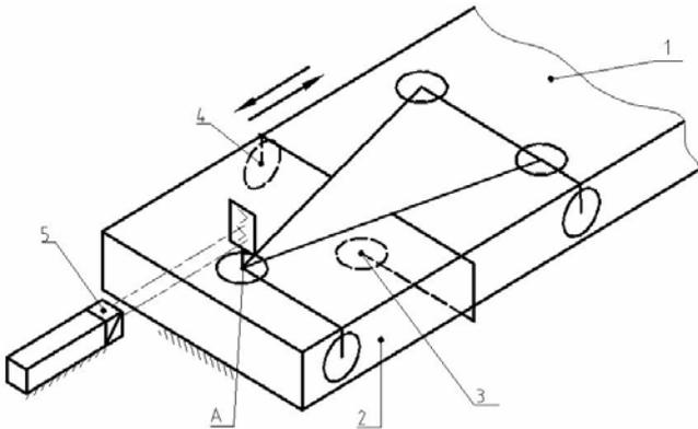
Fig. 1 Unit of linear movement with aerostatic bearings
