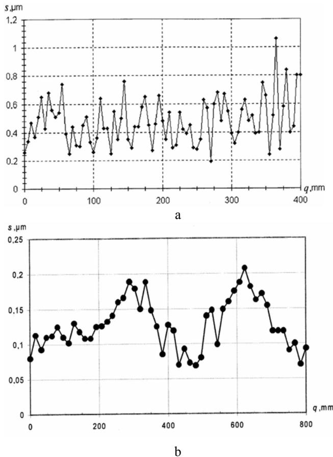
Fig. 2 Dependence of standard deviation in vertical plane on the displacement  $q$  for assemblies with rolling (a) and aerostatic (b) bearings
