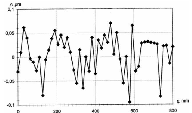
Fig. 8 Deviations of motion straightness errors from low frequency form errors of guideway on the displacement  $q$  for the assembly with aerostatic bearings
