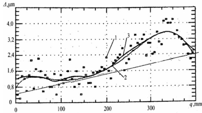
Fig. 5 Deviations of motion straightness (1), their approximation by the algebraic polynomial (2) and guideway form error (3) diagrams for the assembly with rolling bearings
