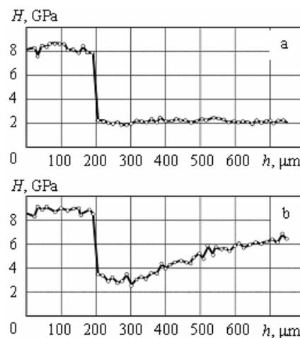
Fig. 1 Depth profiles of the average microhardness in the surface layers of the grade 45 steel samples subjected to EMT after (a) normalization and (b) quenching
