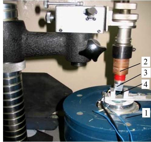
Fig. 1 Experimental setup for parts alignment: 1 – electromagnetic vibrator; 2 – resilient element (metallic bellow); 3 – rectangular (or circular) peg; 4 – part with a slot (in circular parts case – hole bushing)
