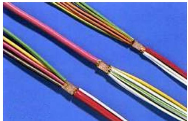
Fig. 1 The ultrasonically welded copper wires
