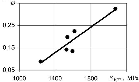
Fig. 5 Relationship between angular coefficient  $\varphi$  and fracture stress  $S_{k,77}$  at the temperature of 77 K
