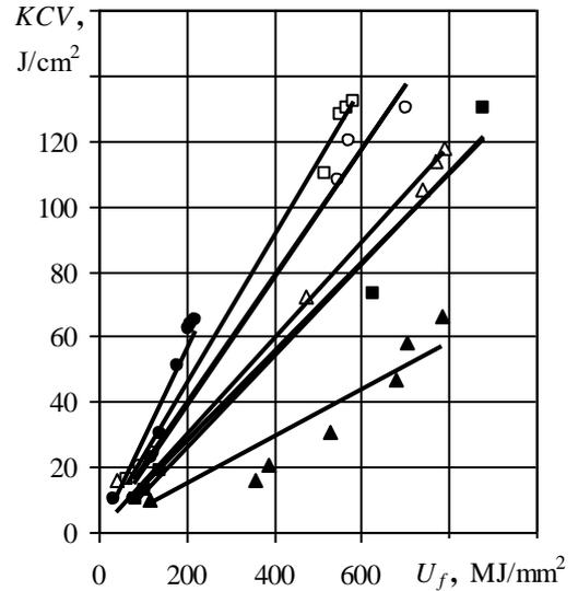
Fig. 4 Relationship between critical indentation energy  $U_f$  and impact strength,  $KCV$ : ● – 17G1S-U, □ – 06G2NAB, ○ – 10G2FB-U, Δ – 10HGNMAYu, ■ – 10G2FB, ▲ – 17GS
