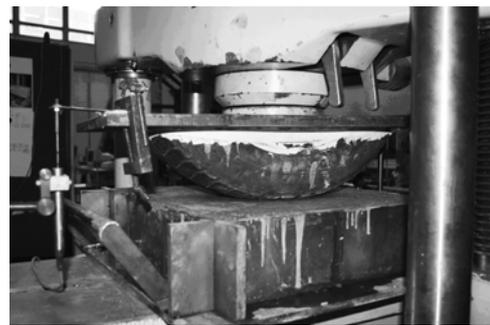
Fig. 7 Pressing cut tire into concrete slab
