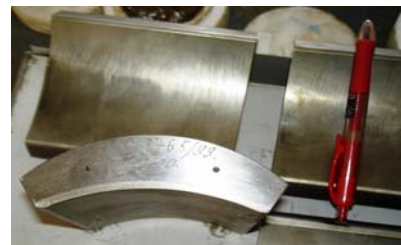
Fig. 3 Damaged 7th tilting-pad journal bearing elements
