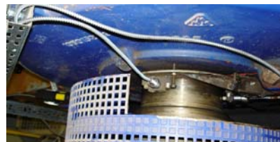
Fig. 2 The blower rotor vibration displacements s_{p-p7} , s_{max7} and shaft position measurement proximity probes location
