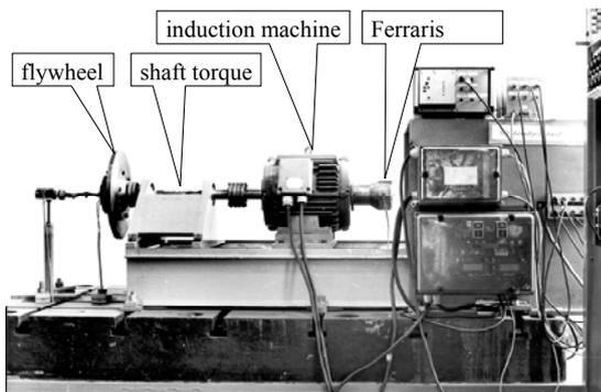
Fig. 8 Test rig to investigate torsional vibrations
