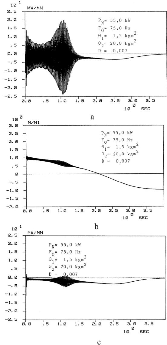
Fig. 5 a - parametric excitation of the shaft torque during reversal; b - simulation of the speed during reversal; c - simulation of electrical torque (reversal)
