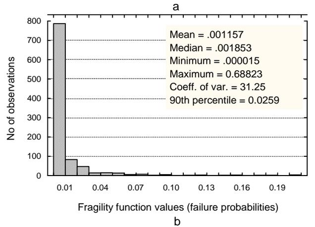
Fig. 4 Visualisation of the simulation results: a – histogram of the values of mean char depths  $d_{mj}(\theta_{\beta k})$ , b – histogram of the fragility function values  $p_j(\theta_{\beta k})$
