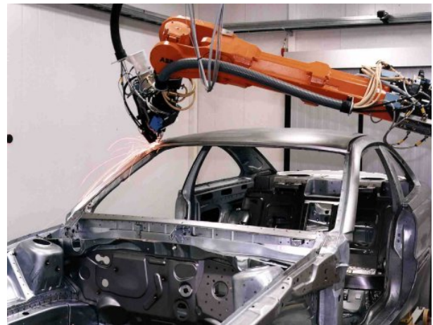
Fig. 2 Laser welding in automotive industry
