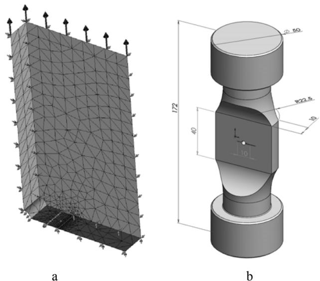
Fig. 3 Three-dimensional (3D) model: a – model of the plate of specific thickness with a crack and FE mesh; b – model coinciding with an experimental specimen
