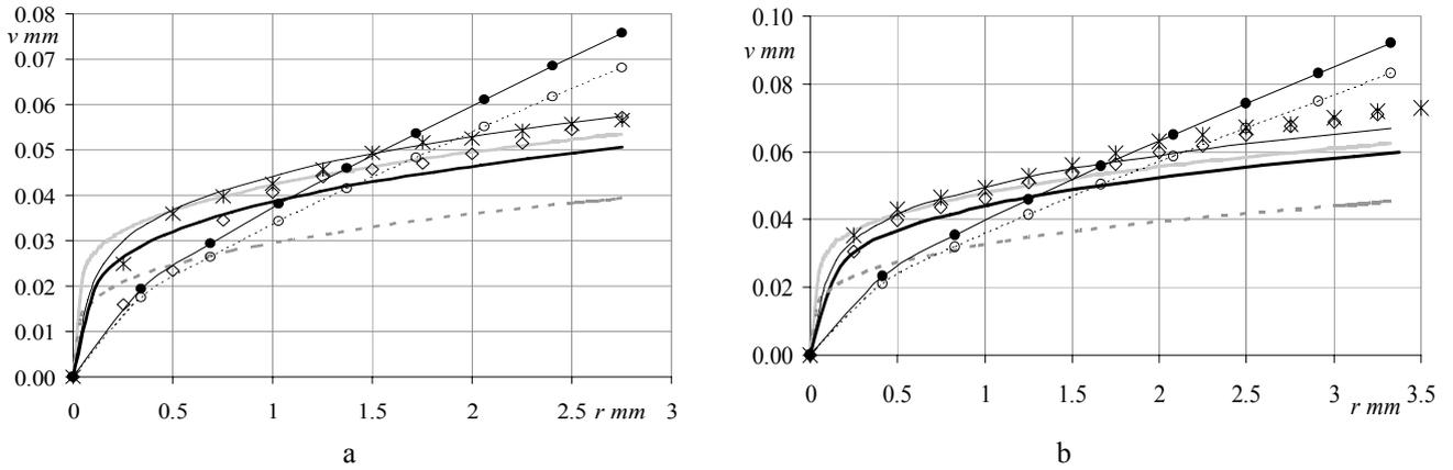
Fig. 7 Curves of the crack opening contour, when the loading  $\bar{\sigma}_{in} = 1$ : a -  $k = 400$  cycles; b -  $k = 600$  cycles
