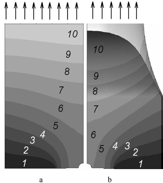
Fig. 4 Comparison of isolines of displacement along y axis, in case of identical loading conditions: a – of the plate of specific thickness; b – of the model imitating the real specimen (the numbers indicate a field coinciding with a specific interval of the displacement)
