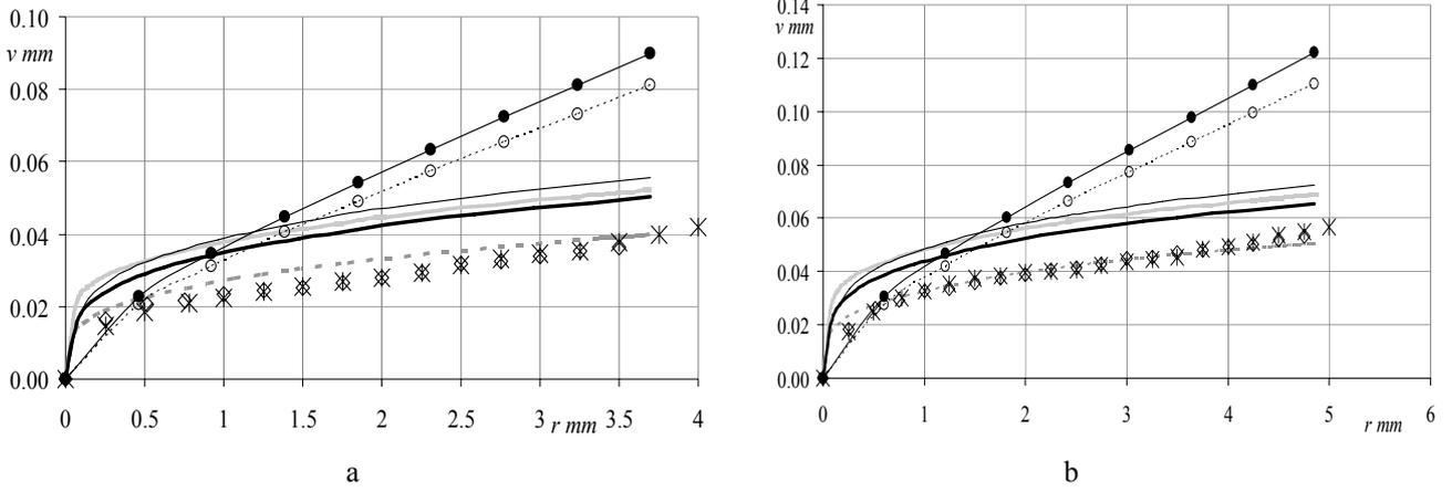
Fig. 6 Curves of the crack opening contour, when the loading  $\bar{\sigma}_{in} = 0.9$ : a -  $k = 4000$  cycles; b -  $k = 5000$  cycles
