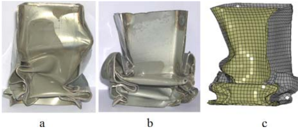
Fig. 4 Specimens used for the experiment: a – after the quasi-static test; b – after the dynamical crushing; c – FEA model after the dynamical crushing
