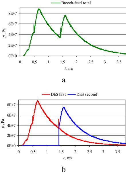
Fig. 3 Time variation of the pressure, acting on the rails: a - Breech-fed regime; b - DES regime
