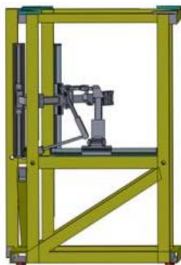
Fig. 1 CAD model of the T3R1 parallel robot
