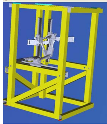
Fig. 6 Parallel robot T3R1 in Matlab/Virtual Reality
