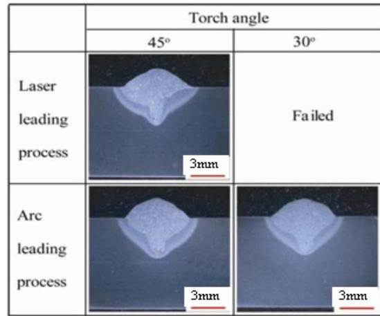
Fig. 7 Influence of the leading process and torch angle; 2 kW laser power, focal point position – 2 mm, MAG current 140 A, voltage 16.5 V and process distance 2 mm
