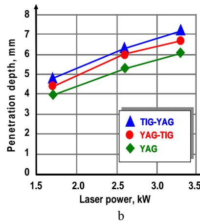
Fig. 8 Shows the comparisons of a) line energy of different welding processes and b) laser power on the penetration depth of bead-on-plate
