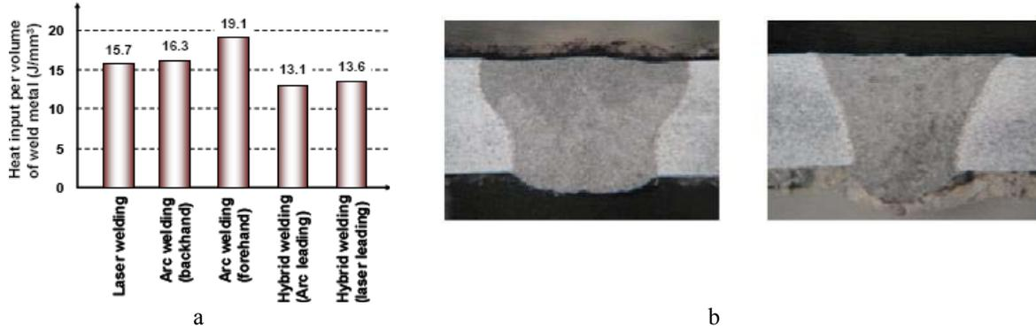
Fig. 6 Shows the comparison of a) Melting efficiency for different welding processes, and b) resulting weld cross-sections with laser leading and arc leading processes
