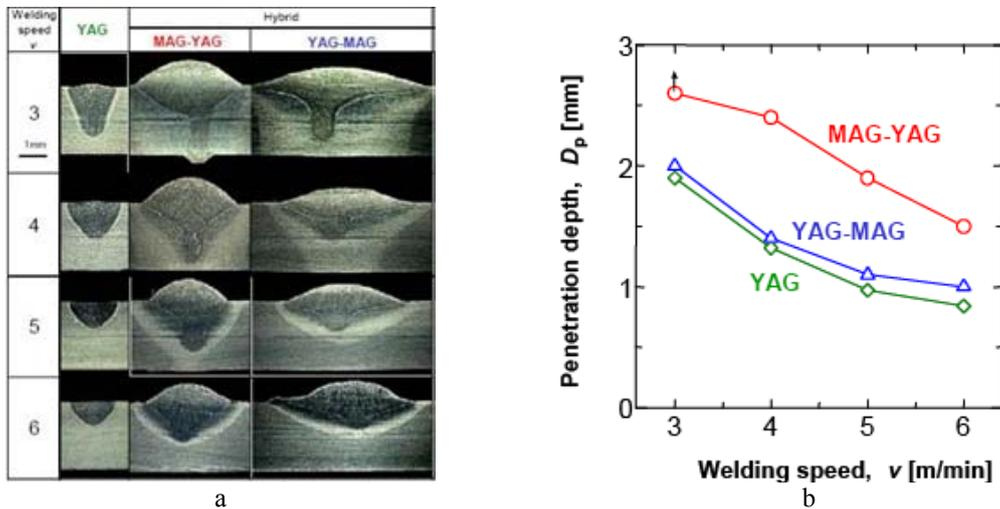
Fig. 2 Effect of the processes as shown by a) a macro-section of weld geometry and b) speed on penetration, with shielding gas Ar + CO<sub>2</sub> (20%),  $I = 200$  A (pulsed MAG), laser power 2.6 kW and 590 MPa high strength steel
