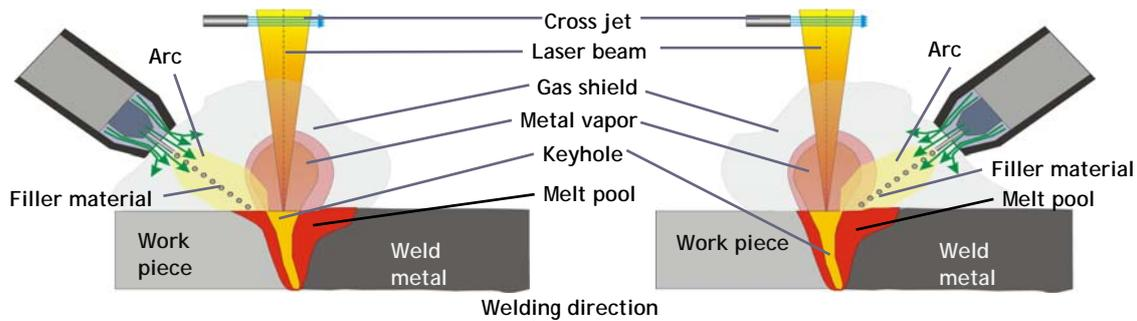
Fig. 1 Schematic representation of hybrid welding with leading arc and leading laser arrangement
