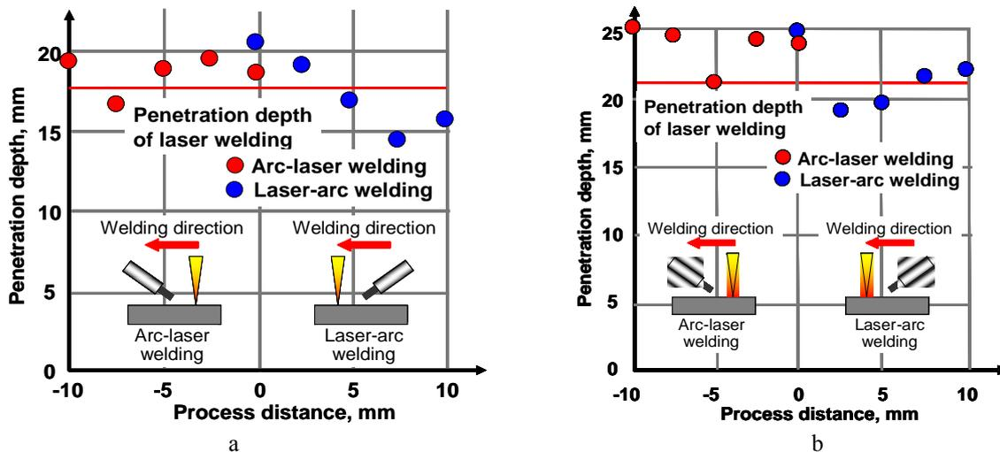
Fig. 10 Effect of process distance on the penetration depths of welds produced in a) a flat position and b) a horizontal position in arc-laser/laser-arc leading hybrid welding with laser power of 30 kW, MIG welding current of 500 A, 47 V and welding speed of 1.02 m/min, bead-on-plate welding
