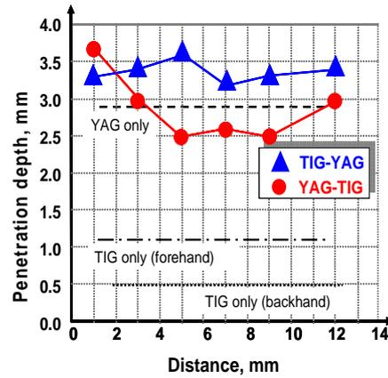
Fig. 9 Effect of distance between the laser beam axis and TIG electrode on penetration depth in Nd:YAG laser-TIG hybrid welding of AISI 304. Thickness 10 mm,  $I = 100$  A,  $v = 0.6$  m/min, focal point position 0 mm, process distance TIG-YAG hybrid 5 mm, YAG-TIG hybrid 1 mm, shielding gas Ar ( $5.0 \times 10^{-4}$  m<sup>3</sup>/s)
