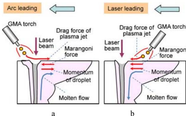
Fig. 4 Driving forces of the molten metal flow for welding directions of (a) leading arc and (b) leading laser.
