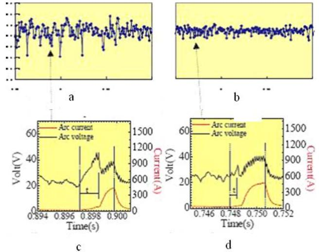
Fig. 5 Influence of welding direction on the variation of voltage and arc current; 5 kW CO<sub>2</sub> laser and a pulse MAG power inclined at 35 degrees, shielding gas 20 l/min via MAG torch, arc pulse frequency 111 Hz, process distance 3 mm and welding speed 3 m/min. The letters a and c represent the leading arc direction with droplet to pulse frequency ratio of 91%, and b and d represent the leading laser direction with droplet to pulse frequency ratio of 100%,
