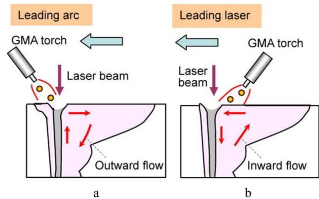
Fig. 3 Schematic diagram of fluid flow in hybrid welding a) of leading arc and b) leading laser
