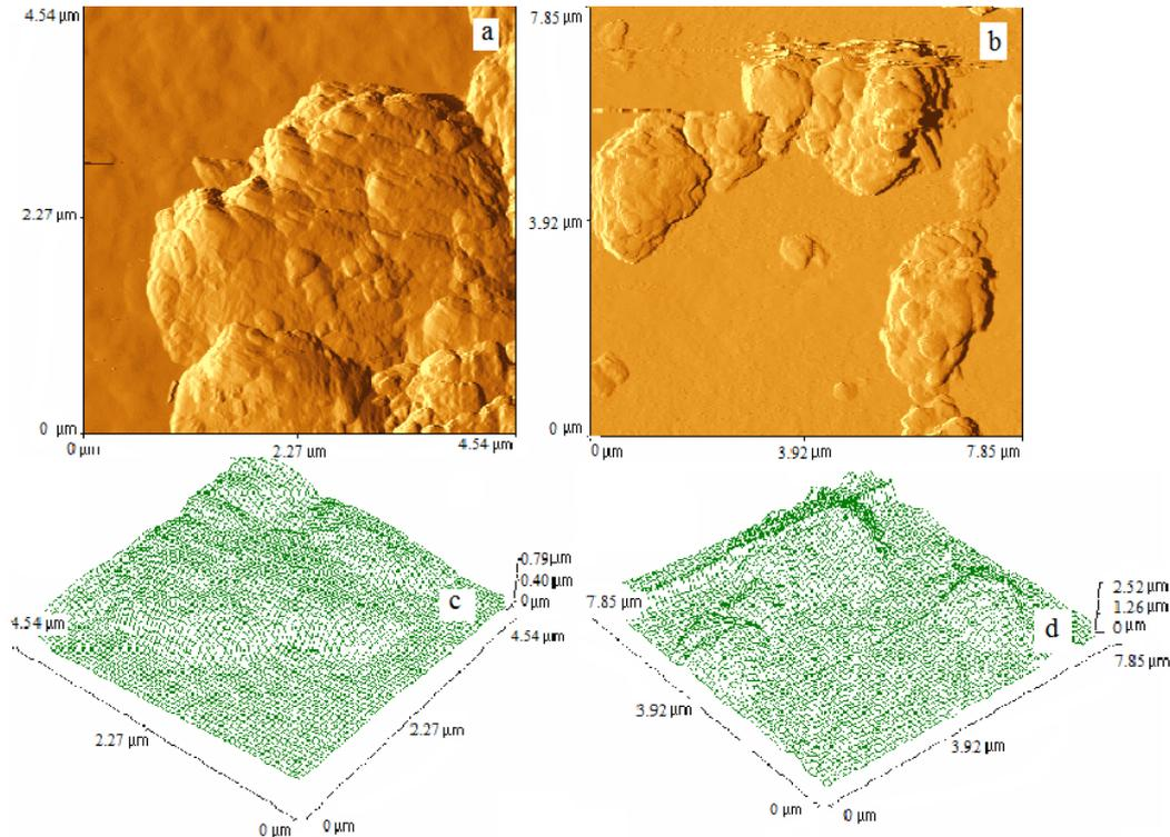
Fig. 6 Surface morphology of debris for WC-Co (a, c) and Cr<sub>3</sub>C<sub>2</sub>-NiCr (b, d)
