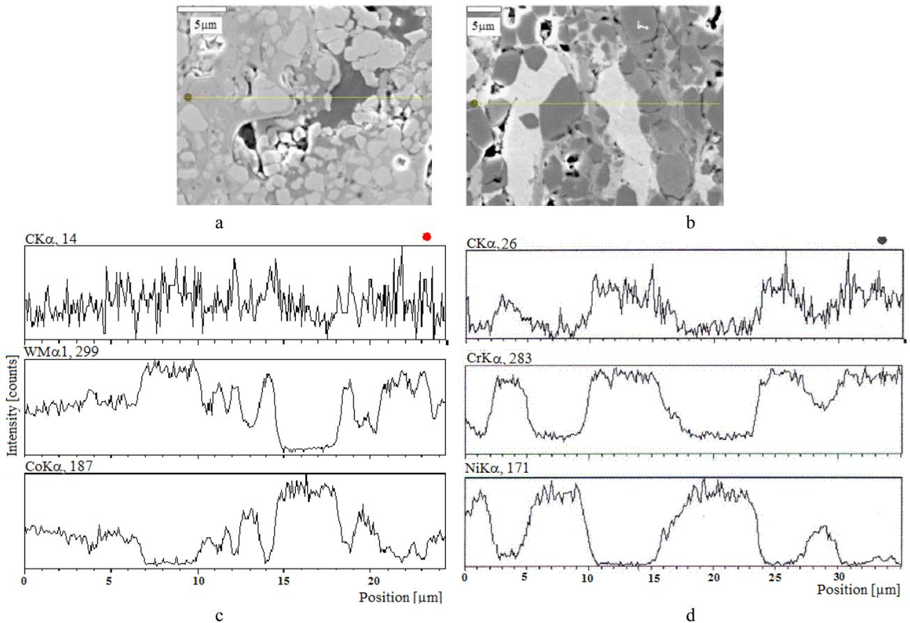
Fig. 4 Microstructure and linear EDX spectra of WC-Co (a, c) and Cr<sub>3</sub>C<sub>2</sub>-NiCr (b, d)
