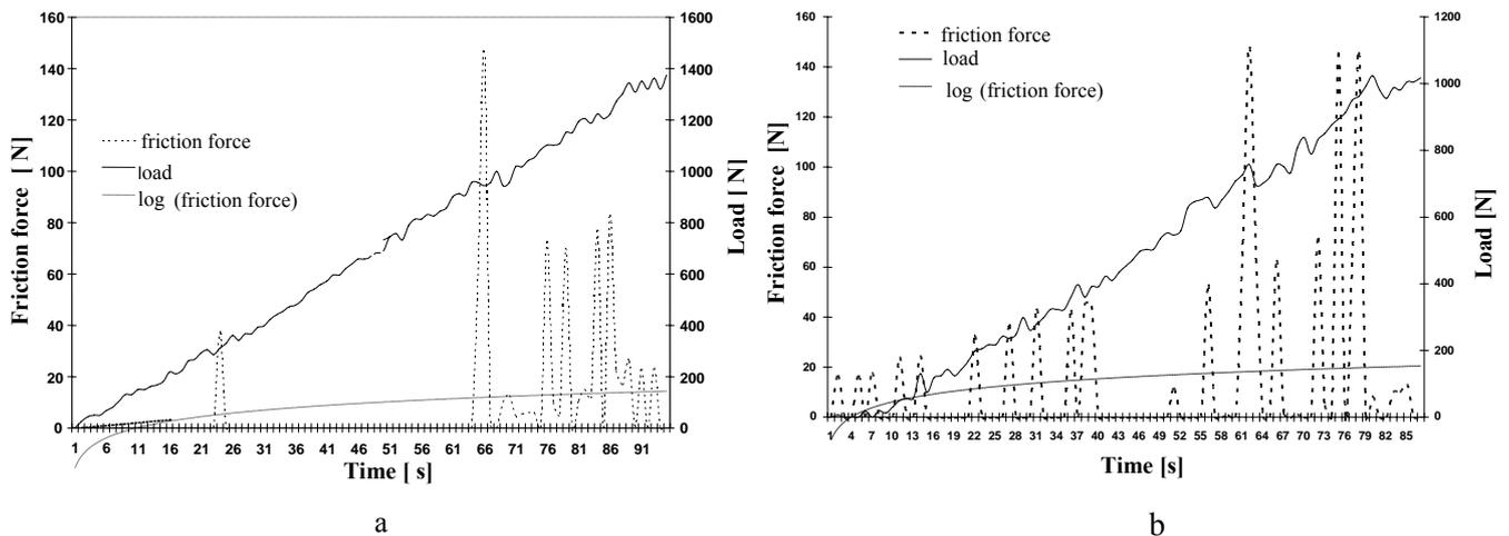
Fig. 5  $F_{max}$  of scuffing resistance for WC-Co (a) and Cr<sub>3</sub>C<sub>2</sub>-NiCr (b)
