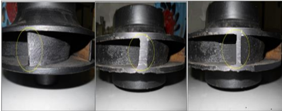
Fig. 14 Pump impellers with different outlet angles: 27°, 30°, and 33°
