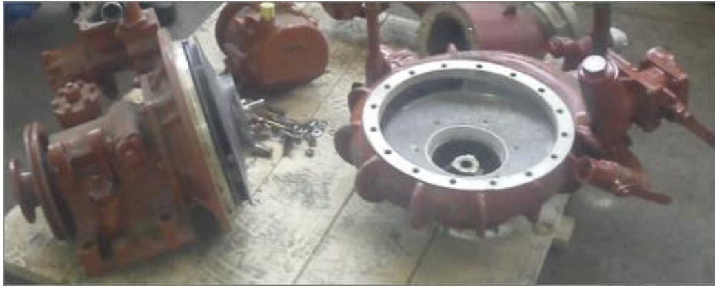
Fig. 13 The used multi-stage pump for the experimentations
