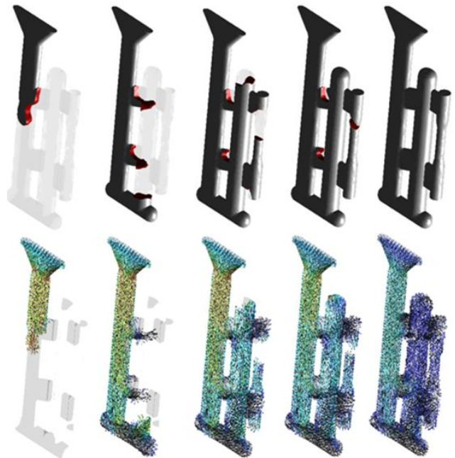
Fig. 15 Vectorial filling analysis degrees in permanent mold of AA 7075 alloy
