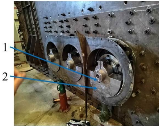
Fig. 14 Vibrating screen rotor end: 1 – transmission shaft, 2 – eccentric rotor
