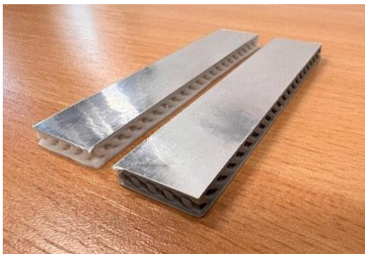
Fig. 3 Liqcreate Composite-X (left, white) and “Phrozen’s Water-Washable (right, grey) samples
