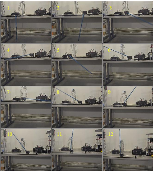
Fig. 17 Sequence of the swing-up and stabilization of the Quanser IP02 SIP system
