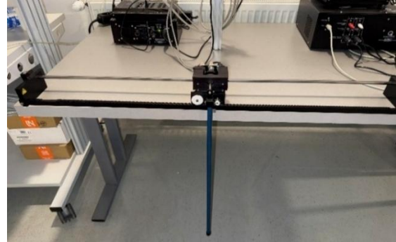
Fig. 14 Single inverted pendulum mounted on the QUANSER IP02 system
