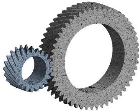
Fig. 9 Mesh Model of Asymmetric Gear Pair
