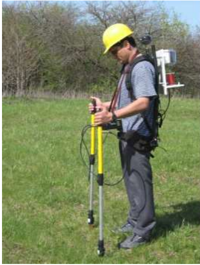
Fig. 1 Inspection on the pipeline route DCVG method [7]
