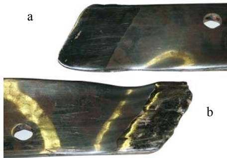
Fig. 8 Front surface welded with high content of carbon and chromium Fe-C-Cr-Si (a) and high content of carbon, chromium, silicon and boron Fe-C-Cr-Si-B (b) hard layers
