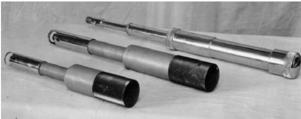
Fig. 8 Dynamic indentation devices, designed in Kaunas University of Technology, for non-destructive evaluation of structures
