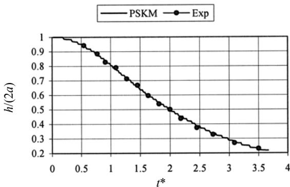
Fig. 2 Quantitative comparison of the numerical results (PSKM) and experimental measurements (Exp). Non-dimensional height of the collapsing water column  $h/(2a)$  versus non-dimensional time  $t^* = t\sqrt{g/a}$
