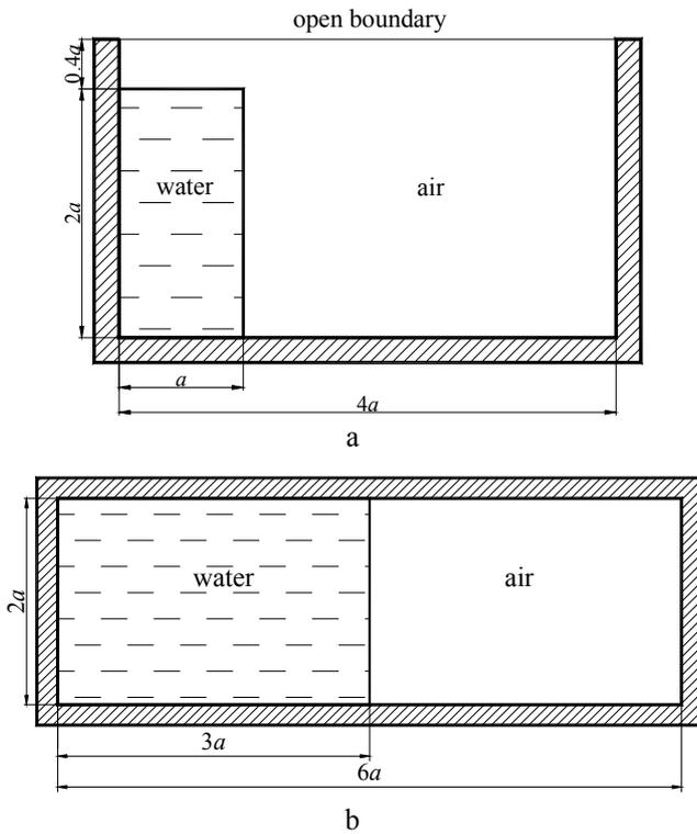
Fig. 1 Geometry of broken dam problems
