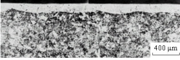
Fig. 4 Micrograph of a longitudinal section of white layer track in normalized grade U7 steel (no zones of thermal interaction of neighbor fragments)
