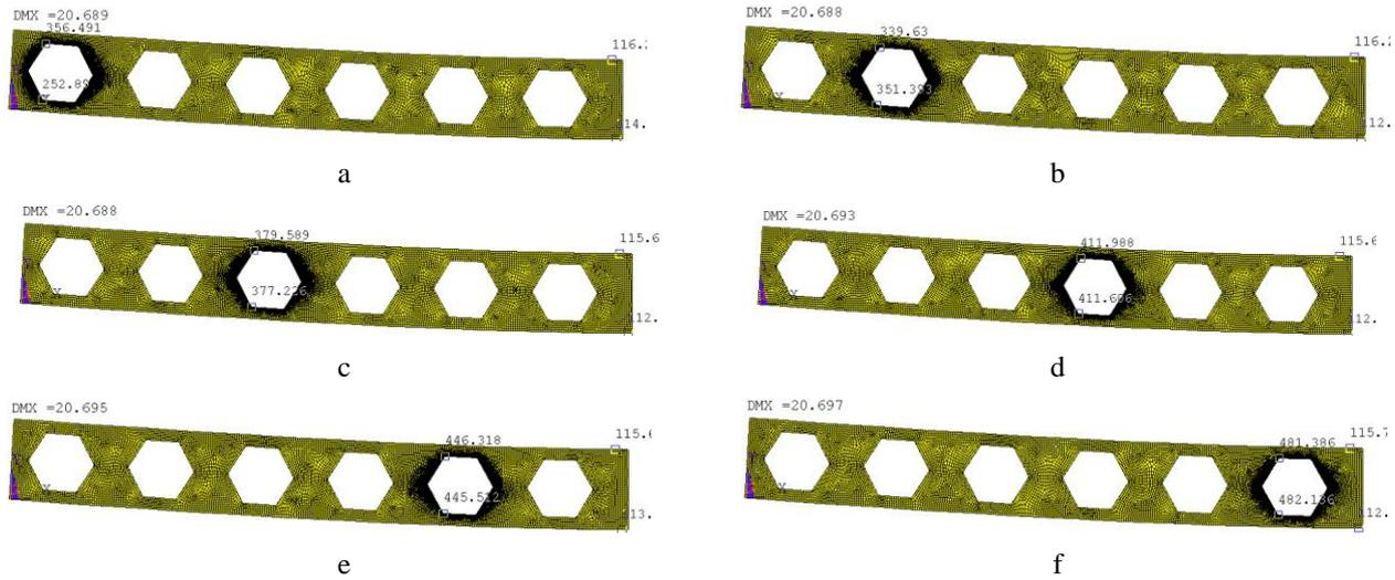
Fig. 6 Stresses in simply supported I-beam 1125-75-1-17-1.52cm-0.7-1 under transverse bending: a - 1st; b - 2nd; c - 3rd; d - 4th; e - 5th; f - 6th holes
