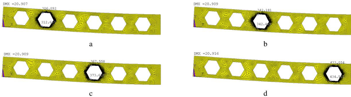
Fig. 4 Stress state of I-beam with dimensions 1125-75-1-17-1.52 cm-0.667-1 under action of concentrated force  $P = 112.25$  kN: a - 2nd; b - 3rd; c - 4th; d - 6th holes
