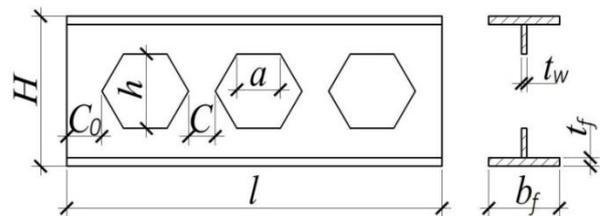
Fig. 1 Calculation scheme of castellated beam
