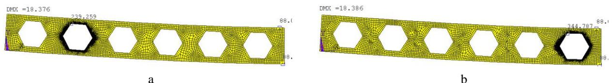
Fig. 8 Stresses in simply supported I-beam 1350-90-1.2-19-1.78 cm-0.7-1 under transverse bending: a - 2nd; b - 6th holes
