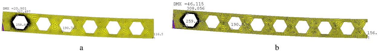
Fig. 3 Stress state near ended hole under constant force in beams  $l-75-1-17-1.52\text{cm}-0.667-1$  of different length: a -  $l = 15H$ ; b -  $l = 20H$
