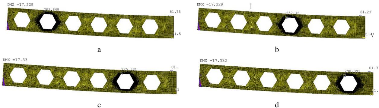
Fig. 5 Stress state of I-beam with dimensions 1350-90-1.2-19-1.78 cm-0.667-1 under transverse bending: a - 2nd; b - 4th; c - 5th; d - 6th holes
