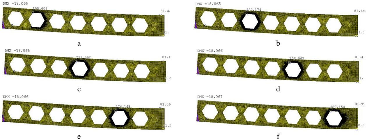
Fig. 9 Stress state of I-beam with dimensions 1350-90-1.2-19-1.78 cm-0.667-0.5 under transverse bending: a - 2nd; b - 3rd; c - 4th ; d - 5th ; e - 6th ; f - 7th holes
