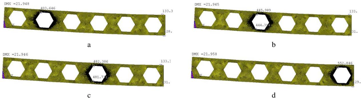
Fig. 7 Stresses in simply supported I-beam 1125-75-1-17-1.52 cm-0.73-1 under transverse bending: a - 2nd; b - 3rd; c - 4th; d - 6th holes
