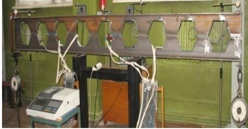
Fig. 11 Test set-up with castellated I-beam model 410-38-0.6-12-1 cm-0.667-1
