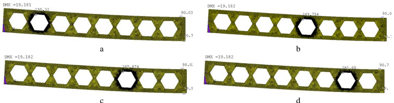
Fig. 10 Stress state of I-beam with dimensions 1350-90-1.2-19-1.78 cm-0.667-0.3 under transverse bending: a - 2nd; b - 5th; c - 6th; d - 7th holes
