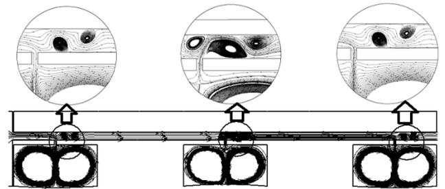
Fig. 6 Streamlines of out-of-phase state for the first arrangement,  $t^* = 0.25$
