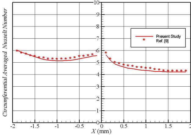
Fig. 4 Variations of circumferential Nusselt number along the micro-channel length
