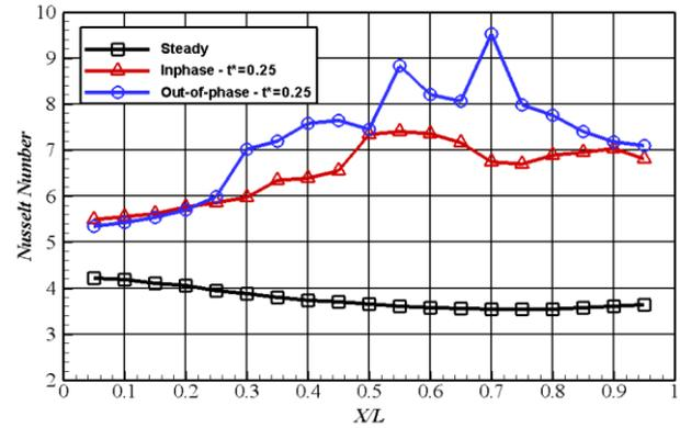
Fig. 12 Variations of Nusselt number over the silicon-water interface wall in the second arrangement of synthetic jets
