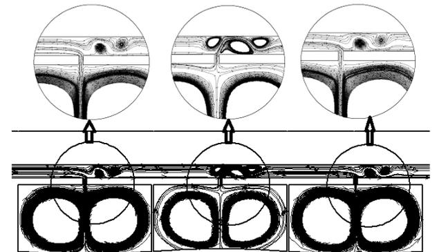
Fig. 8 Streamlines of out-of-phase state for the second arrangement,  $t^* = 0.25$
