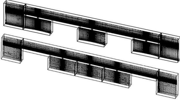
Fig. 2 Arrangement of the synthetic jets along the channel
