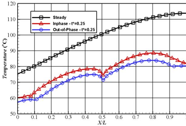
Fig. 9 Temperature variations over the silicon-water interface wall for the first arrangement of the synthetic jets
