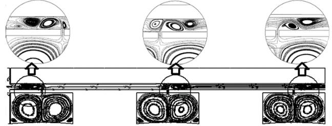
Fig. 5 Streamlines of in-phase state for the first arrangement,  $t^* = 0.25$
