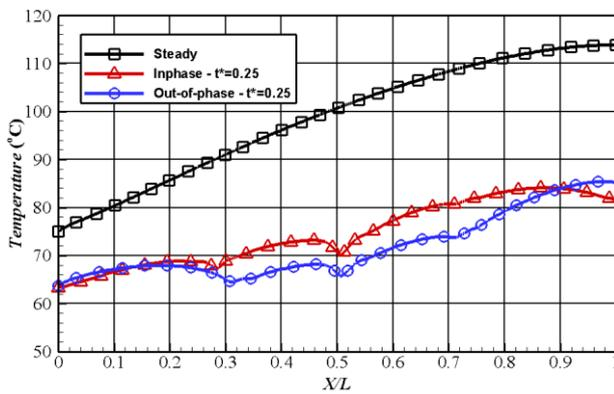
Fig. 10 Temperature variations over the silicon-water interface wall in the second arrangement of synthetic jets
