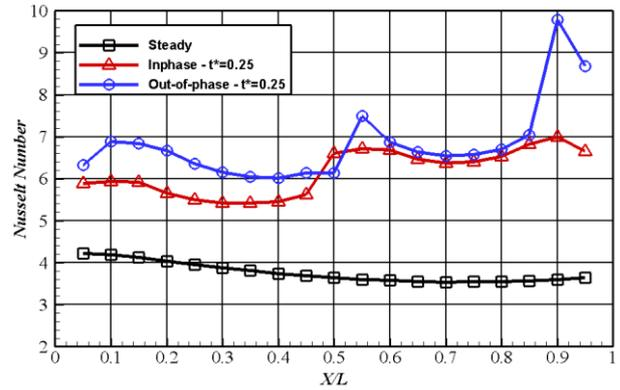
Fig. 11 Variations of Nusselt number over the silicon-water interface wall in the first arrangement of synthetic jets
