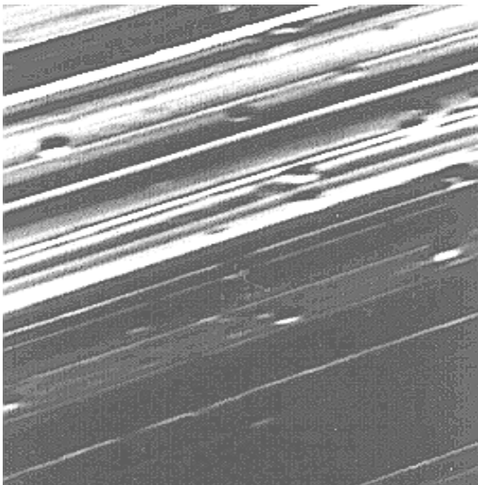
Fig. 13 An example of details of friction surface friction FbA test, load 10 N; lubricant: 3SJ solution in white oil, c = 0.025 \text{ mol/dm}^3
