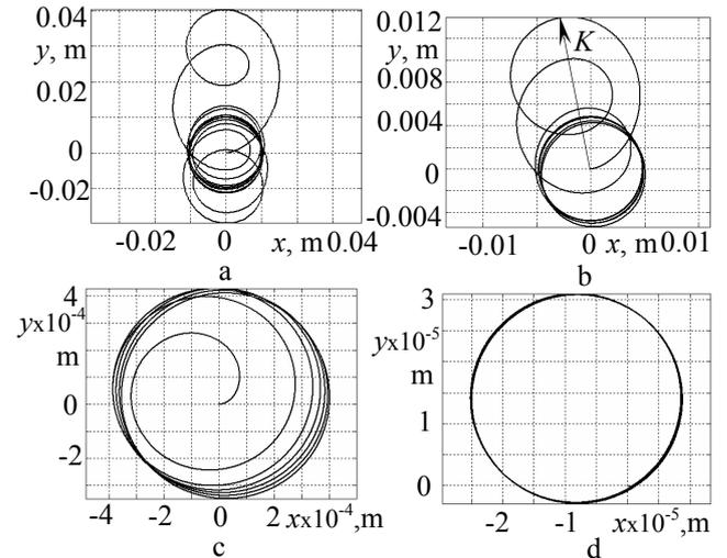
Fig. 4 Character of trajectories on  $xy$  plane, as  $R_e=0.01$  m,  $m=0.01$  m,  $F=5$  N,  $h_x=h_y=0.2$  Ns/m,  $c_x=c_y=10$  N/m,  $\omega=180$  s $^{-1}$ : a -  $\mu=0.01$ , b -  $\mu=0.1$ , c -  $\mu=0.45$ , d -  $\mu=0.63$
