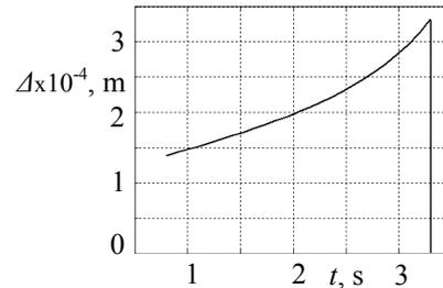
Fig. 19 Change of helix interwinding step, as  $v=0.01$  m/s,  $\omega=60$  s<sup>-1</sup>,  $R_e=0.005$  m,  $c=15$  N/m,  $h_x=h_y=0.2$  Ns/m,  $c_x=c_y=14$  N/m
