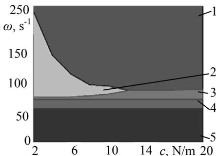
Fig. 8 Zones of motion regimes in coordinates  $c$  and  $\omega$ , as  $R_e=0.005 \text{ m}$ ,  $\mu=0.1$ ,  $h_x=h_y=0.2 \text{ Ns/m}$ ,  $m=0.01 \text{ kg}$ ,  $F=3 \text{ N}$ ;  $c=c_x=c_y$
