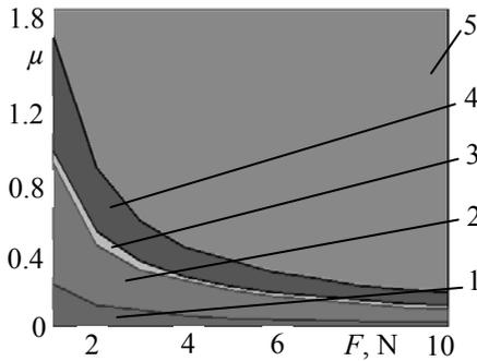
Fig. 5 Zones of motion regimes in coordinates  $F$  and  $\mu$ , as  $\omega=150 \text{ s}^{-1}$ ,  $m=0.01 \text{ kg}$ ,  $R_e=0.005 \text{ m}$ ,  $h_x=h_y=0.2 \text{ Ns/m}$ ,  $c_x=c_y=10 \text{ N/m}$ ,
