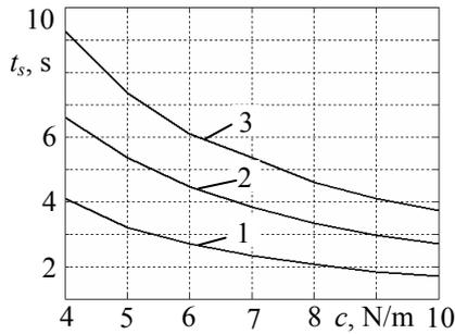
Fig. 15 Dependence of time as part stops on peg's pressing spring rigidity  $c$  and excitation amplitude  $R_e$ , as  $m=0.005$  kg,  $v=0.005$  m/s,  $h_x=h_y=0.2$  Ns/m,  $c_x=c_y=10$  N/m,  $\mu=0.3$ ,  $\omega=50$  s<sup>-1</sup>: 1 -  $R_e=0.005$  m, 2 -  $R_e=0.0075$  m, 3 -  $R_e=0.01$  m
