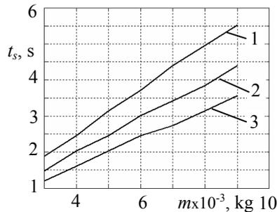
Fig. 17 Dependence of the time the part stops moving both on the bushing's mass  $m$  and friction coefficient  $\mu$ , as  $v=0.01$  m/s,  $R_e=0.01$  m,  $\omega=45$  s<sup>-1</sup>,  $c=15$  N/m,  $h_x=h_y=0.2$  Ns/m,  $c_x=c_y=10$  N/m,  $\omega=45$  s<sup>-1</sup>: 1 -  $\mu=0.2$ , 2 -  $\mu=0.25$ , 3 -  $\mu=0.3$
