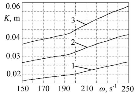
Fig. 10 Dependence of part displacement both on excitation frequency  $\omega$  and amplitude  $R_e$ , as  $\mu=0.1$ ,  $h_x=h_y=0.2 \text{ Ns/m}$ ,  $c_x=c_y=10 \text{ N/m}$ ,  $m=0.01 \text{ kg}$ ,  $F=2 \text{ N}$ : 1 -  $R_e=0.005 \text{ m}$ ; 2 -  $R_e=0.0075 \text{ m}$ ; 3 -  $R_e=0.01 \text{ m}$
