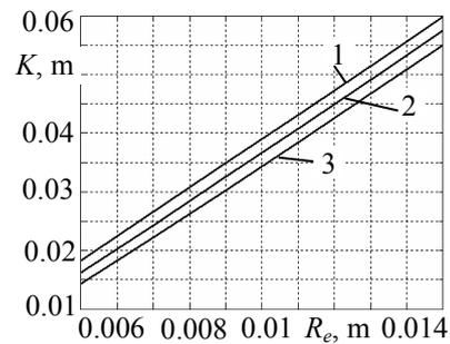
Fig. 9 Dependence of part displacement both on excitation amplitude  $R_e$  and friction coefficient  $\mu$ , as  $F=2 \text{ N}$ ,  $m=0.01 \text{ kg}$ ,  $h_x=h_y=0.2 \text{ Ns/m}$ ,  $c_x=c_y=10 \text{ N/m}$ ,  $\omega=150 \text{ s}^{-1}$ : 1 -  $\mu=0.05$ , 2 -  $\mu=0.1$ , 3 -  $\mu=0.15$
