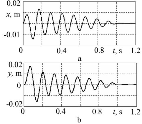
Fig. 13 Character of part vibrations, as  $m=0.01$  kg,  $v=0.08$  m/s,  $c=15$  N/m,  $R_e=0.01$  m,  $\omega=50$  s<sup>-1</sup>,  $\mu=0.01$ ,  $h_x=h_y=0.2$  Ns/m,  $c_x=c_y=10$  N/m; a - along the  $x$  axis direction, b - along the  $y$  axis direction
