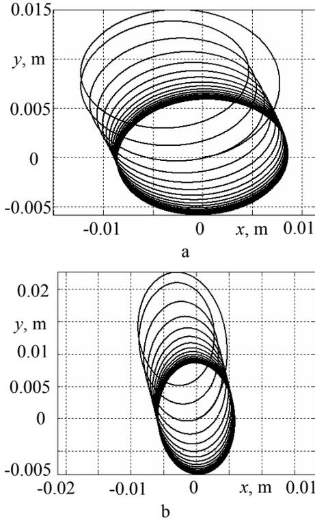
Fig. 11 Part motion trajectory, as plane is vibrated by elliptical mode: a - as amplitude along the  $x$  axis direction is higher than the amplitude along the  $y$  axis direction; b - as amplitude along the  $y$  axis direction is higher than the amplitude along the  $x$  axis direction
