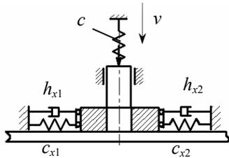
Fig. 12 Scheme used to set varying pressing force
