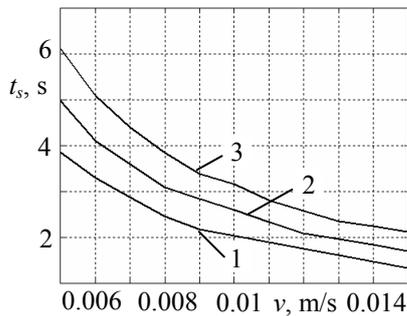
Fig. 16 Dependence of time as part stops, on peg's pressing velocity  $v$  and excitation frequency  $\omega$ , as  $m=0.005$  kg,  $\mu=0.3$ ,  $c=15$  N/m,  $h_x=h_y=0.2$  Ns/m,  $c_x=c_y=10$  N/m,  $R_e=0.01$  m: 1 -  $\omega=45$  s<sup>-1</sup>, 2 -  $\omega=50$  s<sup>-1</sup>, 3 -  $\omega=55$  s<sup>-1</sup>
