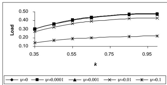
Fig. 5 Variation of load carrying capacity with respect to  $k$  for various values of  $\psi$  where  $\mu = 0.01$
