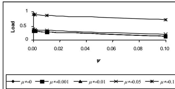
Fig. 6 Variation of load carrying capacity with respect to  $\psi$  for various values of  $\mu^*$  where  $k = 0.4$
