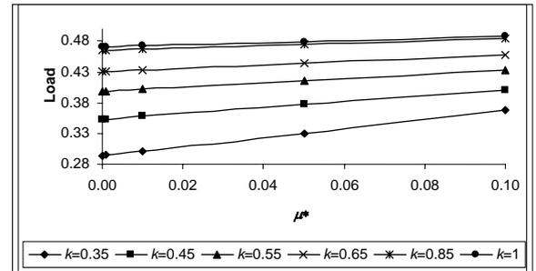
Fig. 2 Variation of load carrying capacity with respect to  $\mu^*$  for various values of  $k$  where  $\psi = 0.001$
