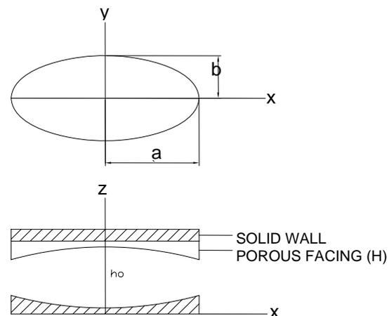
Fig. 1 Configuration of the bearing
