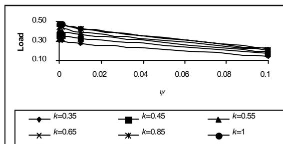
Fig. 7 Variation of load carrying capacity with respect to  $\psi$  for various values of  $k$  where  $\mu = 0.01$
