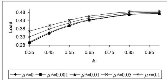
Fig. 4 Variation of load carrying capacity with respect to  $k$  for various values of  $\mu^*$  where  $\psi = 0.001$
