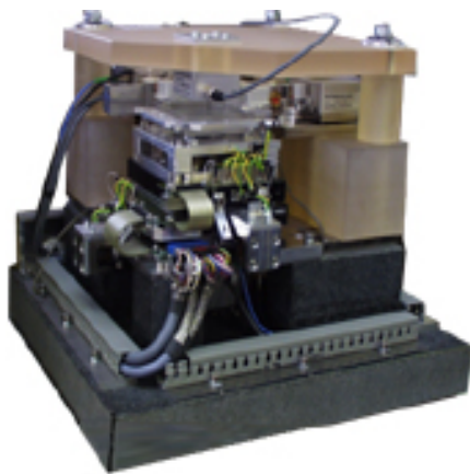
Fig. 1 Scanning probe microscope system in metrology center PTB, Germany [1, 2]
