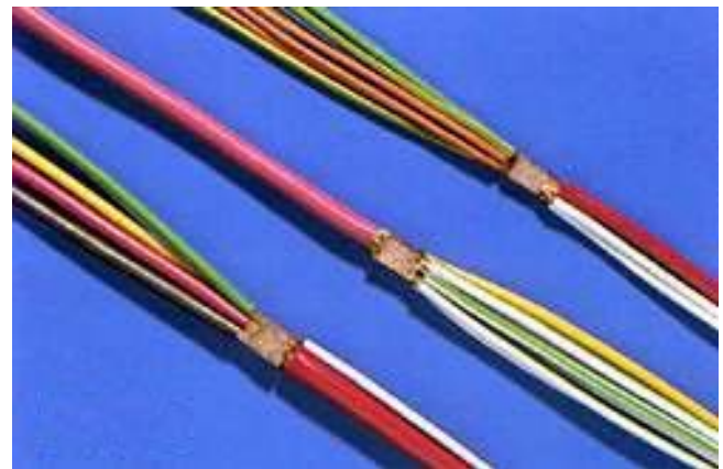
Fig. 1 The ultrasonically welded copper wires
