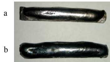
Fig. 4 Single - pass welded layers: a - welded under glass powder, b - under standard AMS1 flux
