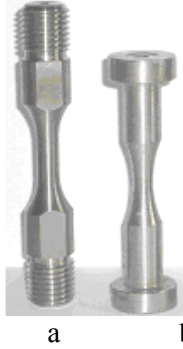
Fig. 1 Specimens used in the investigation: a - cylindrical, b - corset type
