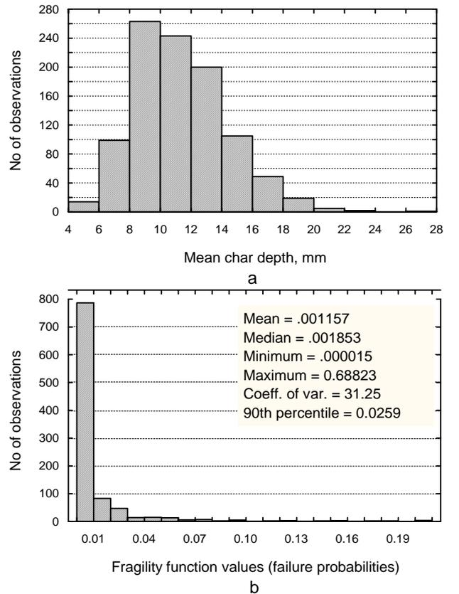
Fig. 4 Visualisation of the simulation results: a – histogram of the values of mean char depths  $d_{mj}(\theta_{\beta k})$ , b – histogram of the fragility function values  $p_j(\theta_{\beta k})$
