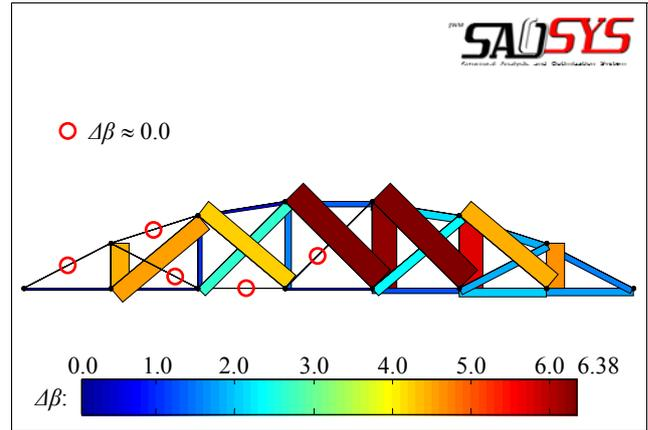
Fig. 8 Outgo diagram of truss elements reliability index
