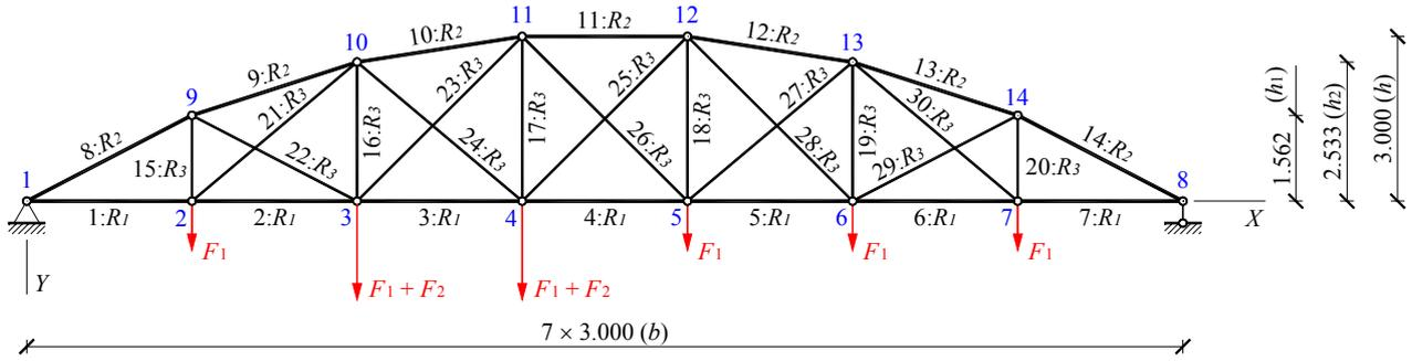
Fig. 6 Truss modeled with LINK1 finite elements
