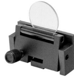
Fig. 3 Photo of universal holder of holographic plate
