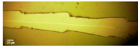
Fig. 4 Scratch tests and scratch views of PVP and Ag/PVP nanocomposites on silicon substrate: a – 20% PVP ; b – scratch view of 20% PVP ; c – 200 mg Ag-NO 3 /20% PVP ; d – scratch view 200 mg Ag-NO 3 /20% PVP
