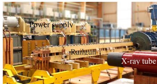
Fig. 1 The ISL-railgun EMA3 railgun facility
