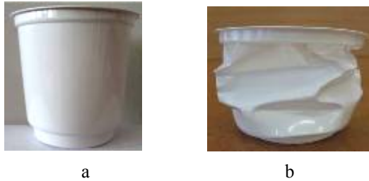
Fig. 8 External view before (a) and after (b) compression of II type (7072/L) of PS package
